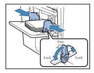
5 Adjust the paper guides according to the envelopes and lock them. 6 Set the Paper Feed Pressure Adjustment Lever to [
