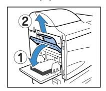
If the paper cannot be removed, while turning Dial C in the direction indicated by the arrow, remove the paper.
