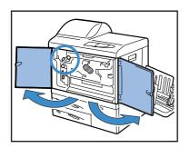
Lift the tab at the left side of the Reversing Path Cover and lock it.
