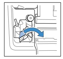
4 Return the tab to its original position and turn the Transfer Lock Lever to the right.
