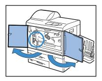
Turn Dial A and remove the paper from the Transfer Roller side.
