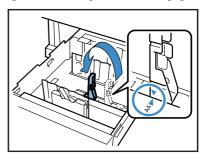
When loading A3/Ledger size paper, do not use the Paper Top Guide. Remove the Paper Top Guide and insert it into the holder in the Paper Feed Tray.
