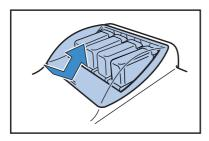
While lifting the lnk Cartridge to be replaced, pull it toward the front side and remove it.
