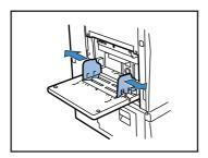
2 Raise the Standard Feed Tray so that the angle from the horizontal plane exceeds 45 degrees and release the stopper roller from the hook.
