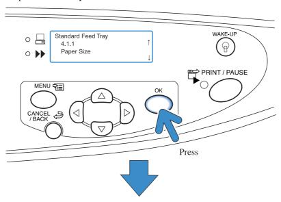
Menu setting can be performed. Press the  $\triangle$  or  $\nabla$  key to select the desired item and press the OK Key.
