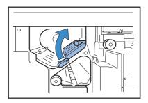
While turning Dial B in the direction indicated by the arrow, remove the paper.
