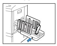
Fold in the Stack Guide (End) outward.
