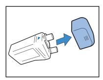
4 Hold the surface of the lnk Cartridge with the ▲ mark up and insert the cartridge until it stops.
