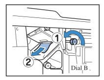
4 If the paper cannot be removed, open the Left Transfer Path Cover and remove the paper.
