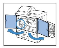
Turn the Transfer Lock Lever to the left and turn down the tab to the right.
