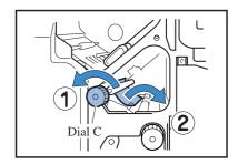
6 Return the tab at the left of the Reversing Path Cover to its original position.
