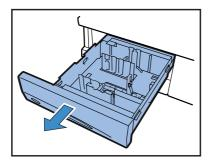
Turn down the Side Guide Locking Levers to the "FREE" positions and spread the guides to the outermost positions.
