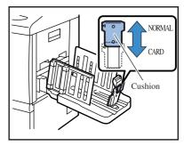
When printing onto paper larger than 320  $\times$  432 mm (12<sup>5</sup>/ $_8$ "  $\times$  17"), fold all the guides.
