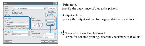
If you click the [Properties] button, you can set the various conditions on the printer driver screen. The settings of [Original image] on the [Main setting] tab and [Paper type] on the [Main setting] tab affect seriously the print quality. When using conditions other than the default settings, click the [Properties] button and adjust the settings.
