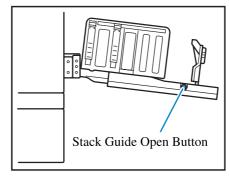
If the button is pressed, the Stack Guides is spread to allow easy removal of prints.
